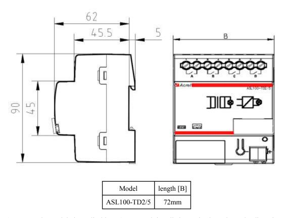
**Installation notes**: the module is applicable to 35mm track installation. It is ok to clamp the dimer into the track. The output terminal is connected with the load and KNX bus is connected with other modules by the bus terminal.
