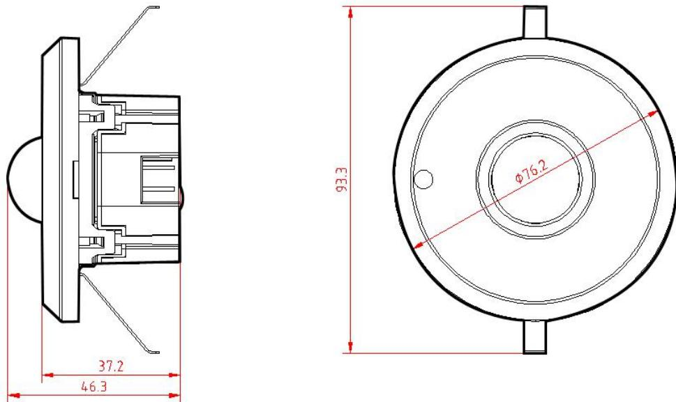
**Installation notes:** the product is easy to install and is embedded. The installation hole size of the sensor is  $\varphi 58\text{mm}$ . During installation, the product is fixed by the leaf springs on both sides. KNX bus is connected by the bus terminal and other modules.
